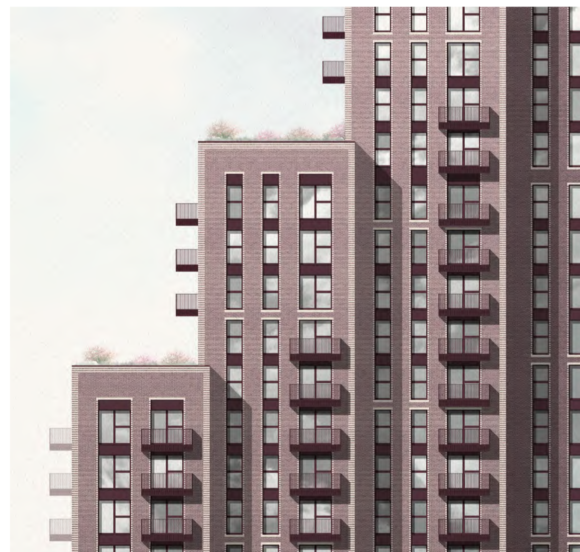
Plum brick with light brick accents around windows and corners. Window frames and balconies matched to brick selection.
